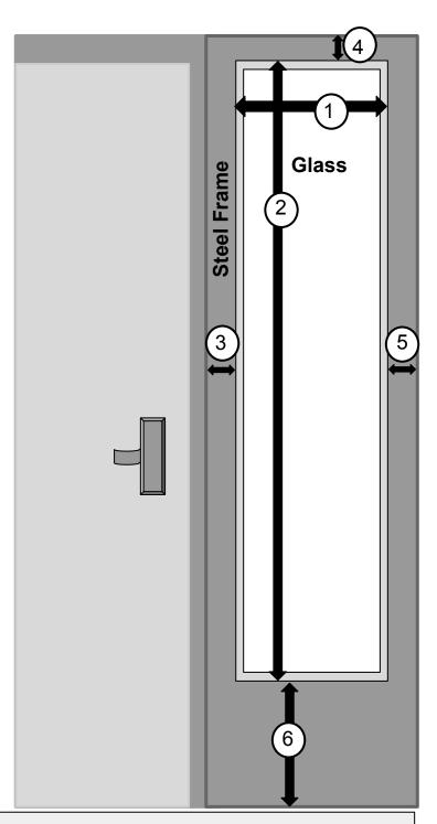
Most sidelight and interior facing school windows have a steel frame which is ideal for Shelter Shutters. If the frame around the glass is not steel, we can provide thin steel adhesive plates to be adhered to the aluminum or non ferrous surface where the shutters magnets meet the metal.
