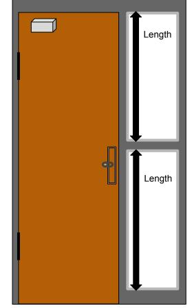
We suggest the top and bottom be made separate. The area next to classroom doors is often a location for waste buckets or other items that may need to be moved to operate the shutter. By making a separate shutter for the bottom, you have options.
